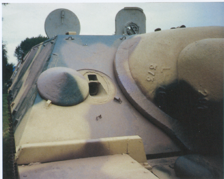
Details evident in this view are the MG42 port, which had a pivoting conical armored cover; the casting marks on the mantlet; the interlocking armor plates; and the fender support bracket.
