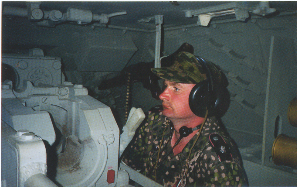
This is the loader's position to the right side of the main gun. He used the breech-operating handle seen here to open and close the breech. More ammunition storage was in the sponson to his right. Above his head is the opening for a non-rotating periscope. The loader operated the vehicle's secondary weapon, the MG42 we see here in travel lock.
