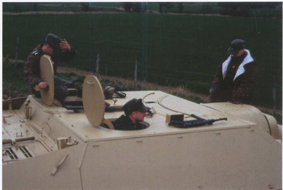
This is a rare view of the top of this vehicle. It is pretty simple and uncluttered, as German vehicles go. To the right front of the loader's hatch is the armored cover for the fixed periscope. The commander's binocular range finder peeks out from the left side of the fighting compartment in front of the commander's hatch. The curved track at the front of the roof accommodates a sliding armored cover that protects the aperture for the gunner's sight when it is not in place. Details to note are the mounting brackets to the rear of the fighting compartment that held the gun cleaning rods. To the bottom right of the photo, you can see the mounting points for shurtzen.
