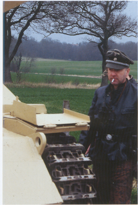
The left front fender showing the hinged mud flap flipped up. You can also see the power cable coming out from the hull and going up over the fender to the headlight mount. The headlight is missing. This shot provides a good view of the track detail. Note the U-Boat leather jacket worn by the vehicle commander.
