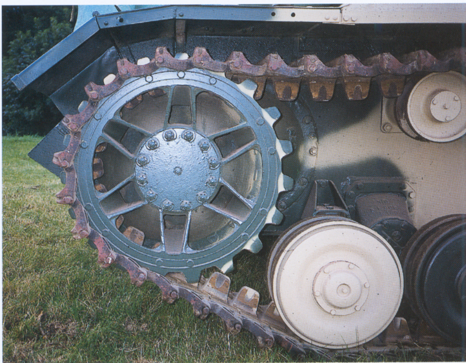
Details of the drive sprocket, track and front fender. Because the vehicle was nose-heavy, the first two road wheel stations utilized all-steel road wheels. The track return rollers were also of steel. Note the wear on the center guides of the track.
