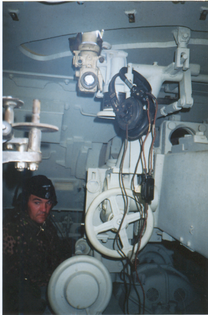
The complete fire control arrangement is seen here to the left of the main gun. The traverse hand wheel is at the bottom. Above that, the elevation hand wheel, then the sight and azimuth indicator – all linked to the main gun. The gunner's headphone and microphone hang on the sight. The driver looks back from his position. Imagine trying to get out of the vehicle quickly! That's why there is an escape hatch. At the upper right, note how the sliding cover for the gunner's sight aperture is latched in the open position.
