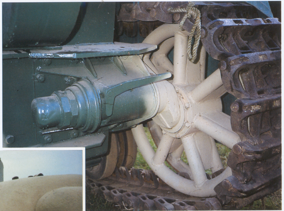
Details of the right idler wheel and housing. The idler wheel could be adjusted to tighten or reduce track tension.
