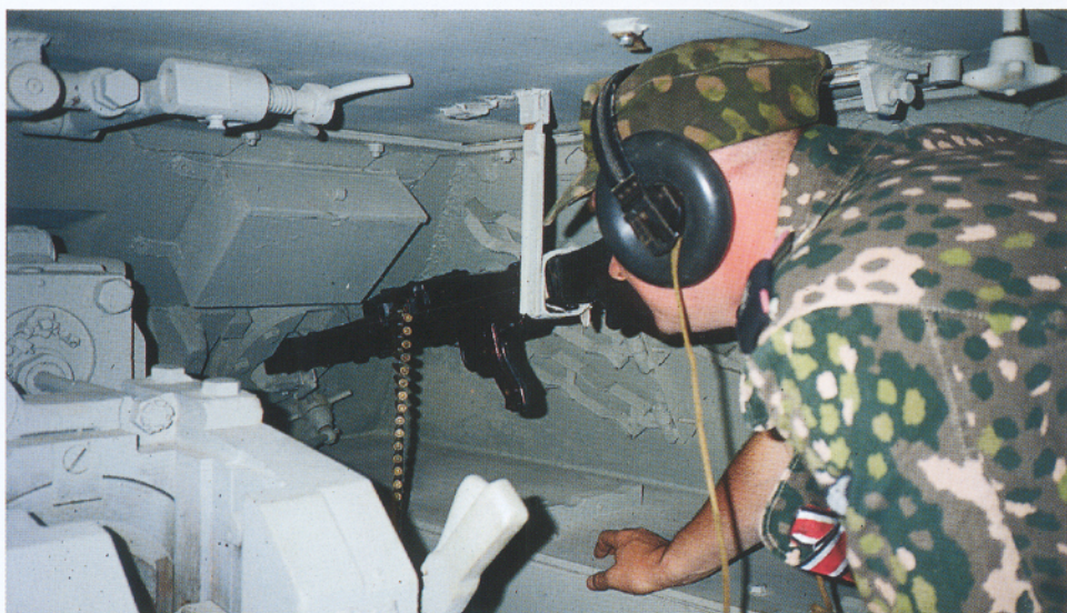
The loader did not have much of a view through a small opening above the machine gun. When not in use, the gun was stabilized with a travel lock that extended from the roof. You can see more brackets for main gun rounds folded up against the side of the fighting compartment.
